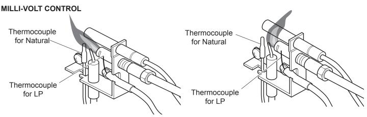
Figure 19 - Correct Appearance of Pilot Flame
